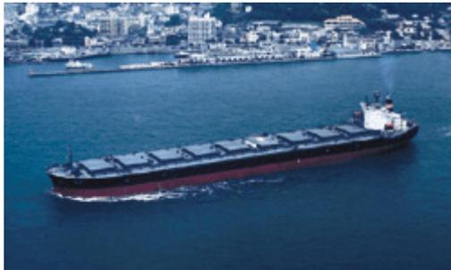
the work horses of the fleet, these transport raw materials such as iron ore and coal. Identifiable by the hatches raised above deck level which cover the large cargo holds.
