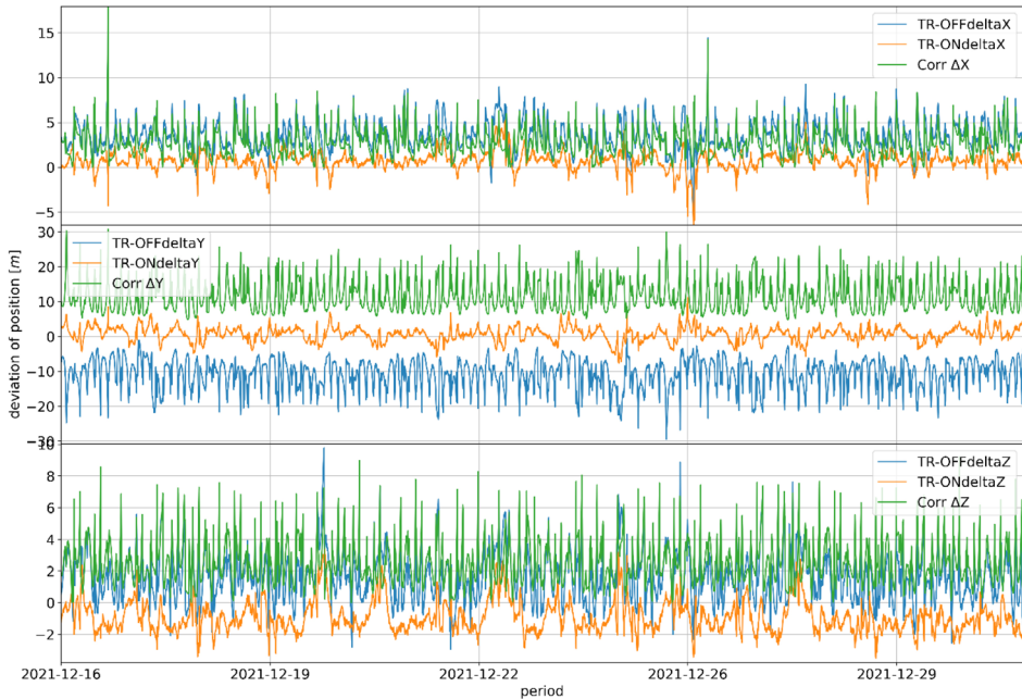
Figure 1. Trends in tropospheric correction and tropospheric error values for GNSS station at Christmas Island, Australia in the period 16 – 31 December 2021.
