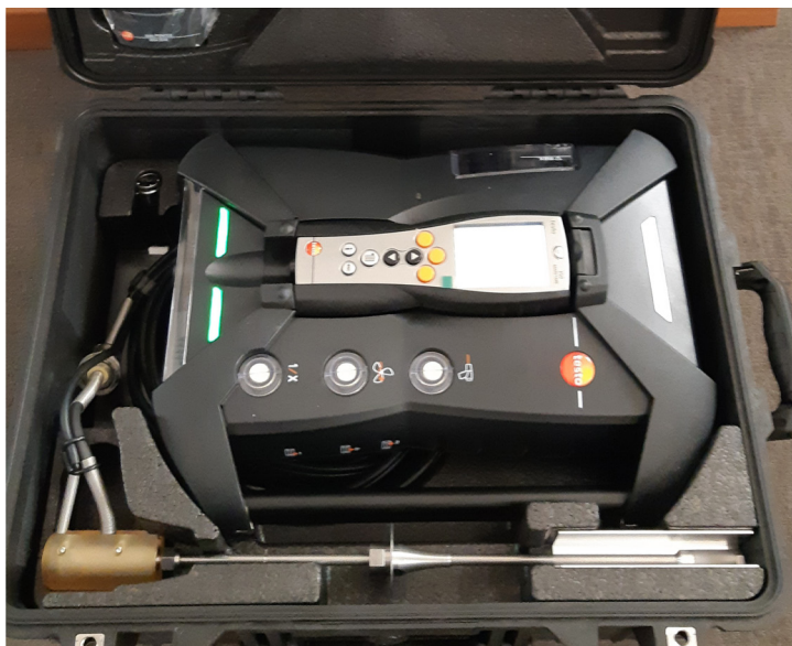
Figure 1. Testo 350 Maritime flue gas analyser.
