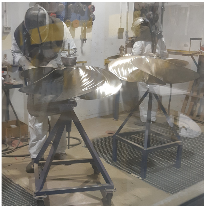
Figure 4. Propeller shape modification.
