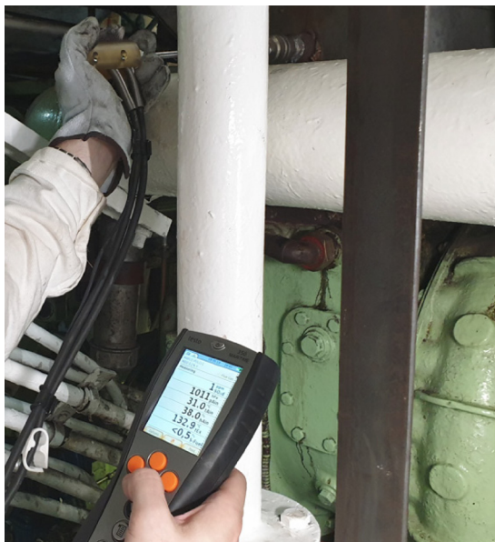
Figure 1. Sampling point for measuring exhaust gases.
