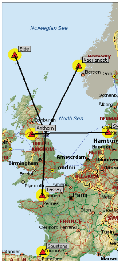
Figure 5 Relevant European Loran-C stations for prototype eLoran.
