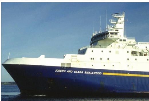
Figure 4 MV Joseph and Clara Smallwood installation shows radar used with RadarFix (second from top of mast).
