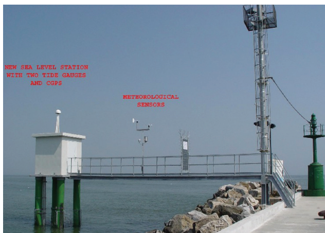
Figure 3. The Porto Garibaldi reference station set-up
